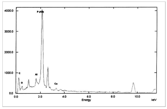
Figure 8 Remains microanalysis shows the presence of high amount of Ca and P.
