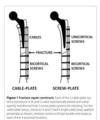
were inserted from the underside of the plate holes, such that the mounts protruded beyond the top surface of the plate to provide access for the Luque wire. A double Luque wire was inserted into 4 proximal wire mounts and then tensioned by manual twisting. Bicortical screw fixation was used to secure the plate distally, as described earlier.
