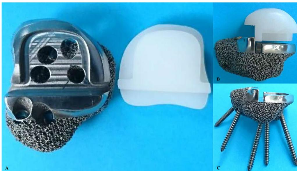
**Fig. 3** The fabrication of the 3D-printed custom-made modular talus prosthesis. **A, B** Screw holes are pre-set in the titanium alloy parts for screw insertion. The UHMWPE part and the titanium alloy parts were connected according to the "snap-fit" design. **C** The screws are evenly distributed
