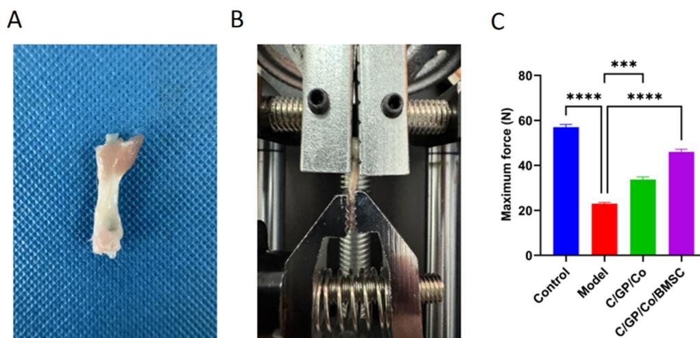
**Fig. 6** Biomechanical evaluation of the Achilles tendon. **A** Tendon samples, including the calf muscle, Achilles tendon, and calcaneus. **B** Tendon mounted on a biomechanical testing machine. **C** Maximum tensile strength of the four groups. Data are expressed as mean  $\pm$  SD ( $N=3$ ). \* $P < 0.05$ , \*\* $P < 0.01$ , \*\*\* $P < 0.001$
