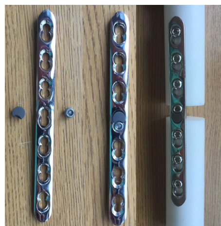
Fig. 1 The left panel shows details of the threaded screw hole insert compatible with the LC/DCP system. The center panel shows the placement of the screw hole inserts on the plate. The right panel shows the configuration of the LC/DCP plate and screw hole inserts mounted on a synthetic UHMW block to simulate fracture fixation
