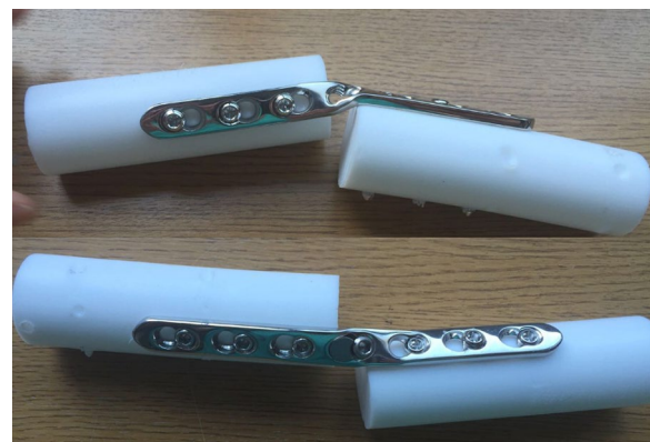
Fig. 4 Top panel: LC/DCP plate without screw hole inserts with torsional torsion at the screw hole. Bottom panel: In the LC/DCP plate with screw hole inserts, rotational fracture was observed between two screw holes rather than a single hole with a lower rotational deformation
