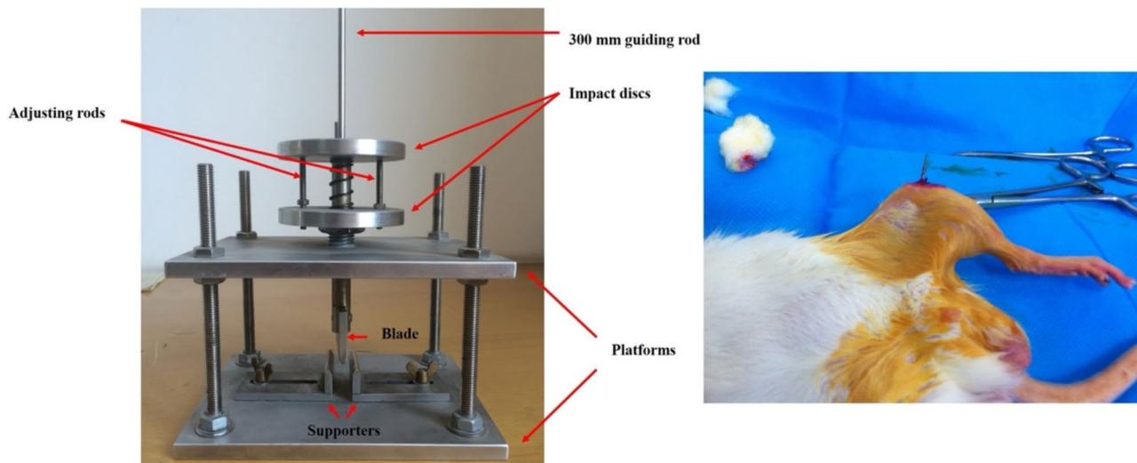
**Fig. 1** Self-designed three-point bending system and intramedullary pinning in rats. Left: The custom-built three-point bending system, showing its key components for controlled fracture induction. Right: The surgical procedure for intramedullary pin fixation in rats before fracture induction
